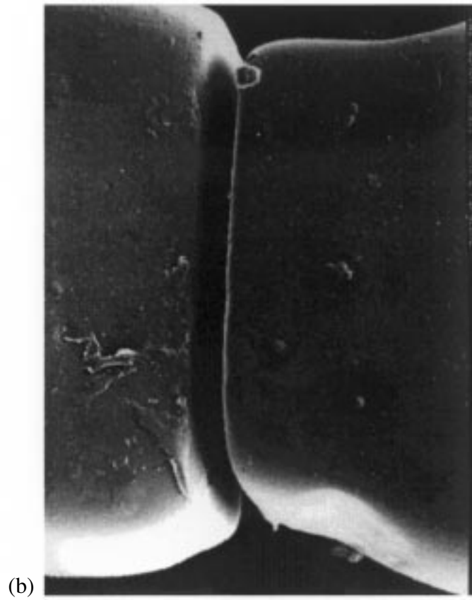
Figure 4 SEM of the (a) uncoated and (b) poly(2-chloroparaxylylene)-coated stent.
